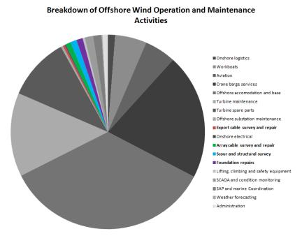
**Figure 3:** Breakdown of offshore wind operations and maintenance activities. The coloured segments (also in bold in the legend) denote activities that are wholly or mostly involved in subsea. Source: Adapted from The Crown Estate Guide to offshore wind O&M, this is based on a 500MW wind farm.
