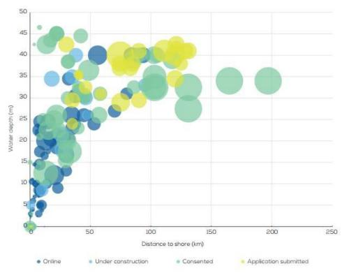
**Figure 5:** Average water depth, distance to shore of bottom-fixed, offshore wind farms by development status. The size of the bubble indicates the overall capacity of the site. Source: WindEurope
