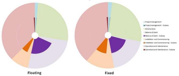
Breakdown of the lifetime cost of an example offshore wind farm
