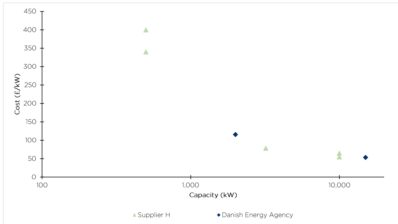
Figure 3: Cost per kW of electric boilers at different capacities. Please note that the horizontal axis is plotted on a logarithmic scale.
