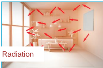
Fig. 1: Infrared light generates heat at the objects (rather heating the air) via radiation. Source: Surya Heating
