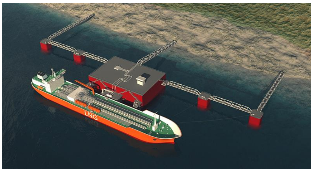
Figure 5-2 Gravifloat LNG receiving terminal (Ref 105)
