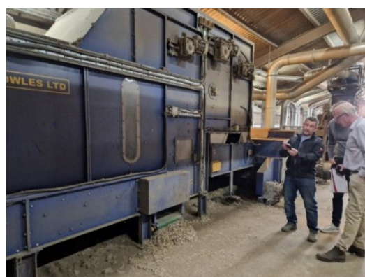
Fig 26 Decortication equipment at East Yorkshire Hemp
