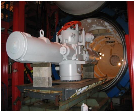
Subsea Actuator being loaded into Hyperbaric Chamber
