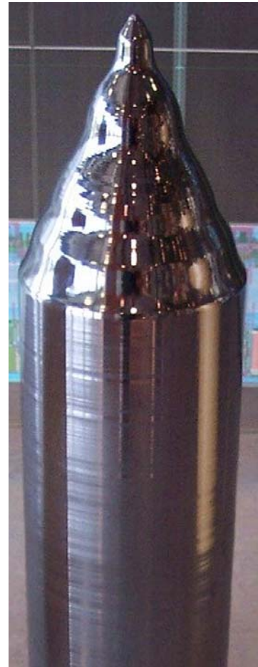
Figure 17: Raw Silicon boule grown from a liquid melt
