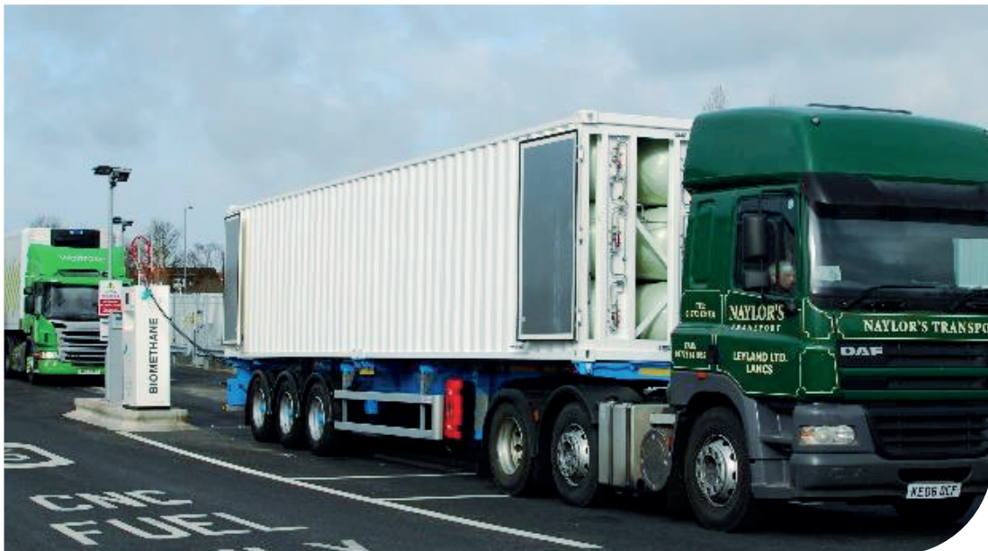
Containerised refuelling system being refilled at public fuelling station. CNG cylinders visible.
