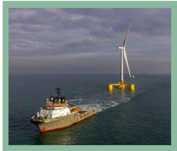
Figure 22 - Source: Boskalis Manta Anchor handler in tow off the coast of Aberdeenshire
