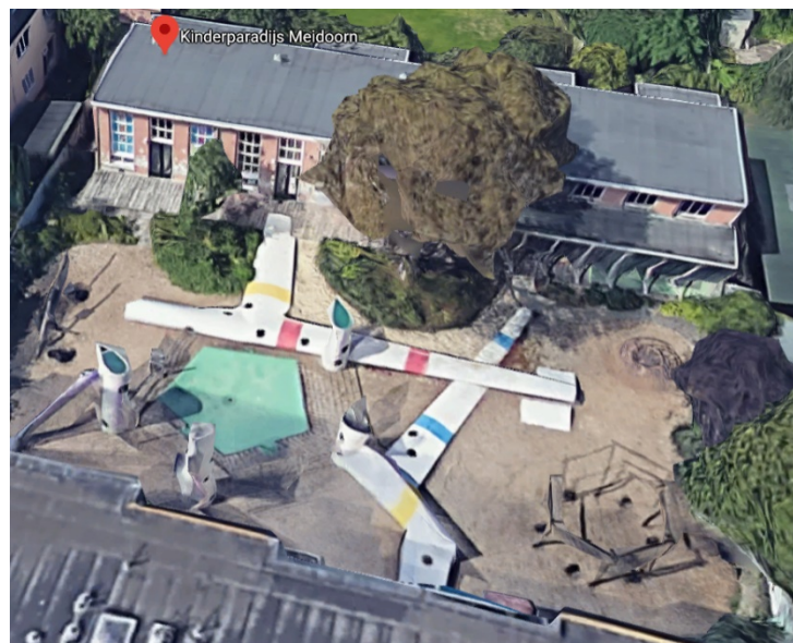
Figure 5 Google maps screenshot from Meidoorn playground in Rotterdam, Netherlands with decommissioned HAWT turbine blades. Straight and curved shapes of VAWT blades offer more versatility towards housing and shelter construction options.
