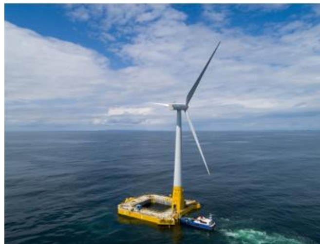
Figure 3.22 Damping Pool – Ideol [33]
