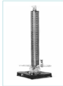
1896: mercury sphygmomanometer Inflatable cuff connected to glass manometer
